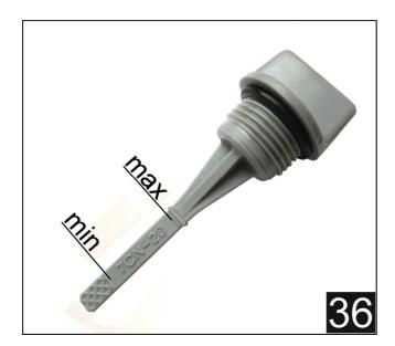
To restore the oil level use the same type of lubricant already present in the engine.
